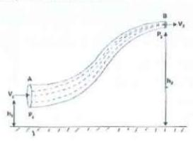
Consider a tube AB of varying cross-section through which an ideal liquid is in streamline flow.
