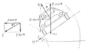
Consider a car of weight mg going along a curved path of radius r with speed v on a road banked at an angle  $\theta$ . The forces acting on the vehicle are
